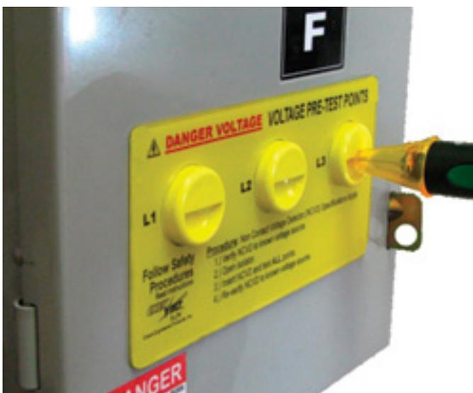
Reliable operation of the NCVD depends upon its ability to complete a capacitive circuit between the tested wire and ground. Without a good path to the power-source ground, the device will not operate reliably. To avoid this pitfall, a voltage portal should only be used on electrical systems where the power source has the ground or neutral connected to earth ground.
