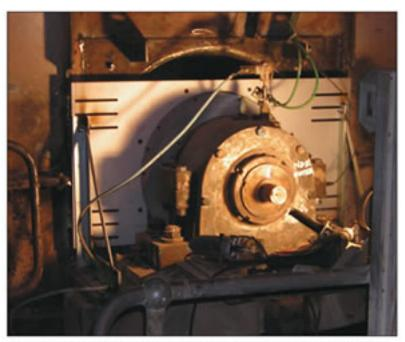
Continual particulate buildup on this kiln pre-heater ID fan rotor (and repeated unscheduled shutdowns to deal with it) impacted Castle Cement's ability to meet production demand. A new balancing system, capable of withstanding the harsh conditions surrounding the unit, now continuously monitors vibration levels and makes rapid corrections while the fan is running.
