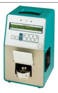
Grabner's MiniFlash is a flash-point tester with a continuously closed cup that requires only 1mL of sample to function. According to the company, it is the first such instrument that doesn't test with an open flame, allowing it to be operated safely and without supervision. Flash point testing within the MiniFlash was developed according to ASTM D6450 and D7094, which give results equivalent to ASTM D56, D93 or ISO 2719, and are used worldwide with a wide range of substances.
