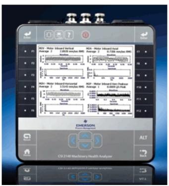
Emerson Process Management has introduced the CSI 2140 Machinery Health Analyzer, the next generation of its portable tool for analyzing machinery vibration to detect potential
