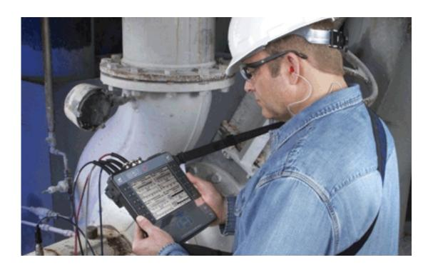
The CSI 2140 Machinery Health Analyzer is a complete tool for assessing and preserving mechanical-equipment health.
