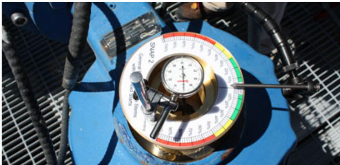
**This new, non-intrusive diagnostic tool makes the job of quantifying critical thread wear faster and easier than in the past.**
