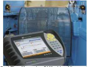
**Real-Time Measuring Of Machine Alignment Changes**
